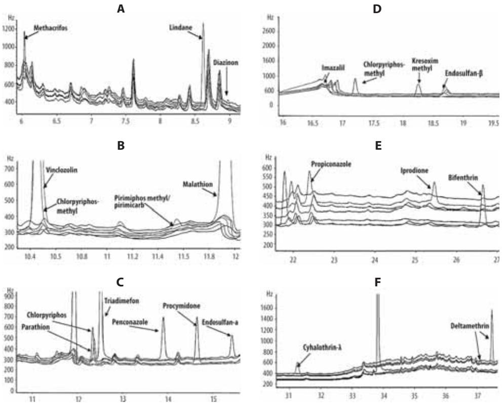
**Figure 1.** Chromatogram in 6 time segments (A to F) of 22 of the 28 analytes in wheat flour at fortification level equal to the limit of quantification ( $LOQ_m$ ). Injection splitless column DB-5MS, detector ECD.
