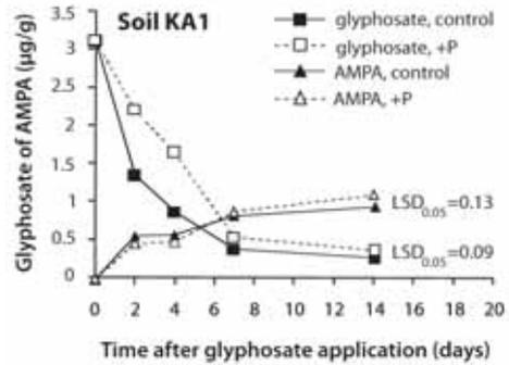
**Figure 7.** Dissipation of glyphosate and accumulation of AMPA in soil KA1 amended or not with 0.3 g/100 g of superphosphate fertilizer.
