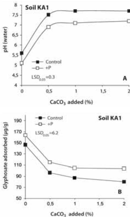
**Figure 5.** Effect of 0,3 g/100 g of superphosphate, added to KA1 soil which had previously been limed with increasing amounts of  $\text{CaCO}_3$  (0, 0.5, 1 and 2), on soil pH (A) and glyphosate adsorption (B).
