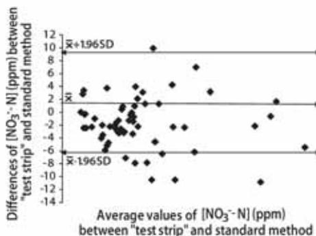
**Figure 2.** [NO<sub>3</sub><sup>-</sup>-N] (ppm) differences between the methods vs. average values of the methods for each composite soil sample. ( $\bar{x}$  = mean of the differences and SD = standard deviation).
