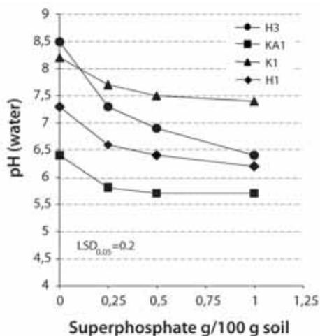
**Figure 4.** Effect of the superphosphate amendment (at three levels equivalent to 220-880 ppm P) on the pH of the four soils.
