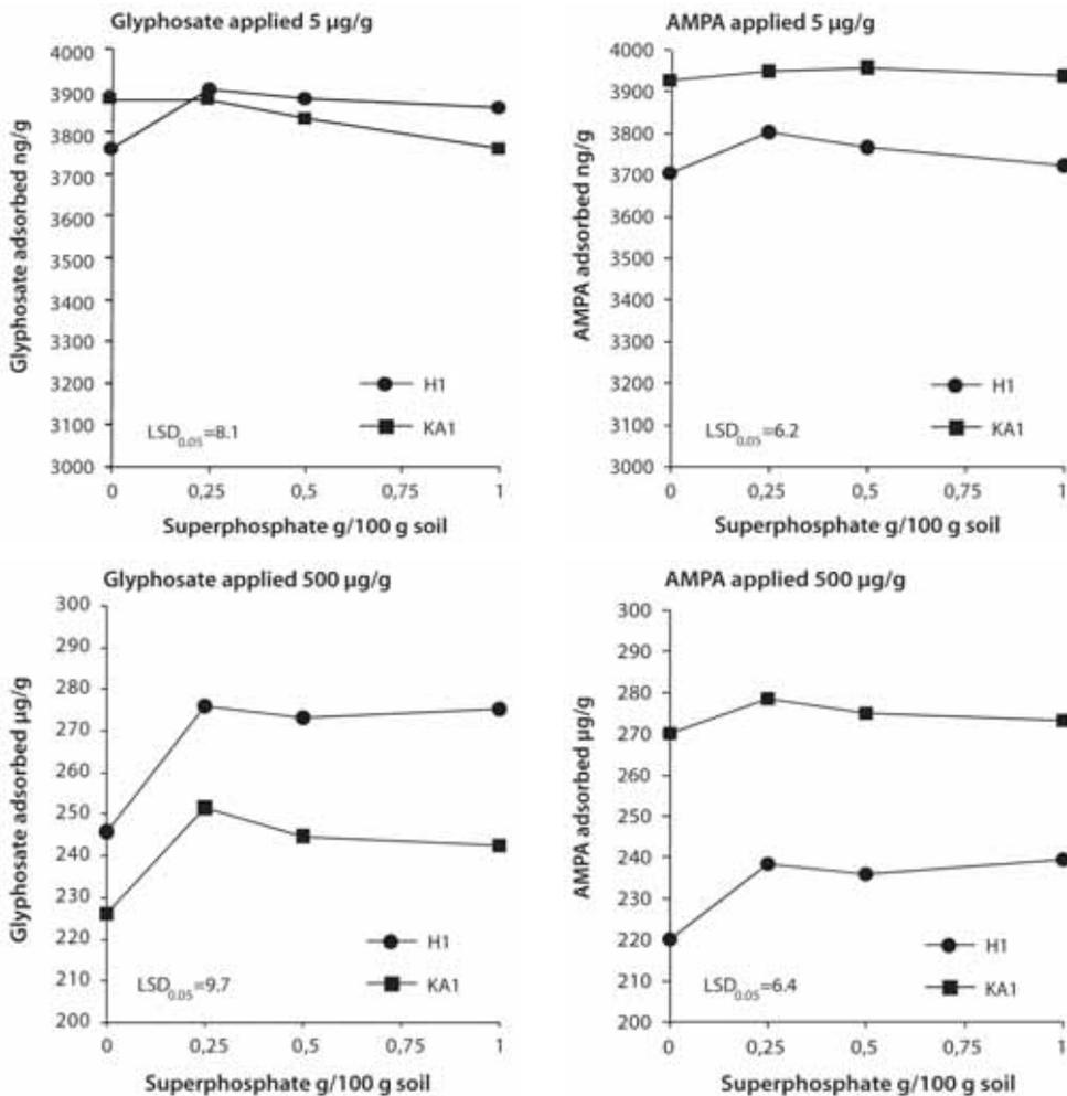
**Figure 2.** Glyphosate and AMPA adsorption on KA1 and H1 soil samples that had been previously amended with the indicated amounts of superphosphate and let to equilibrate for 5 days. Glyphosate and AMPA adsorption was measured by batch equilibration experiments utilizing 10 ml/g of solutions at the proper concentrations to supply the indicated amounts of each chemical.
