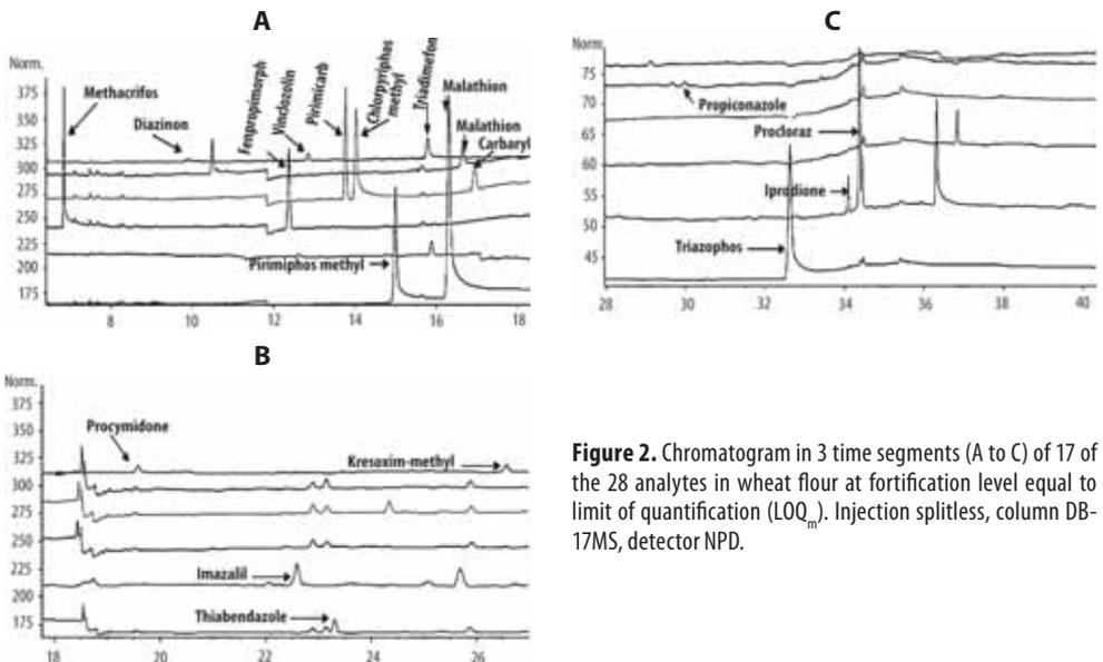
**Figure 2.** Chromatogram in 3 time segments (A to C) of 17 of the 28 analytes in wheat flour at fortification level equal to limit of quantification ( $LOQ_m$ ). Injection splitless, column DB-17MS, detector NPD.
