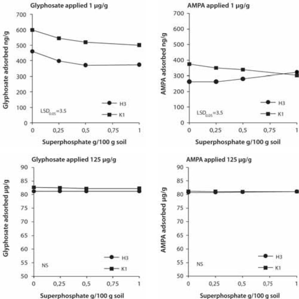
**Figure 3.** Glyphosate and AMPA adsorption on K1 and H3 soil samples that had been previously amended with the indicated amounts of superphosphate and let to equilibrate for 5 days. Glyphosate and AMPA adsorption was measured by batch equilibration experiments utilizing 10 ml/g of solutions at the proper concentrations to supply the indicated amounts of each chemical.
