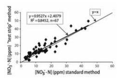
**Figure 1.** Regression analysis between the "test strip" and the standard method and the line of agreement (y=x) between the methods.
