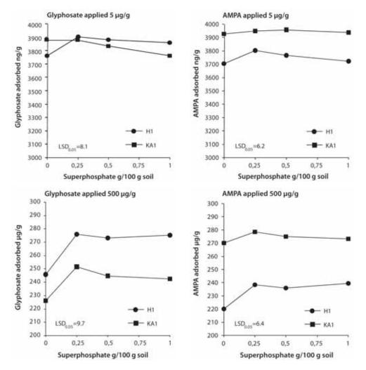
Figure 2. Glyphosate and AMPA adsorption on KA1 and H1 soil samples that had been previously amended with the indicated amounts of superphosphate and let to equilibrate for 5 days. Glyphosate and AMPA adsorption was measured by batch equilibration experiments utilizing 10 ml/g of solutions at the proper concentrations to supply the indicated amounts of each chemical.
