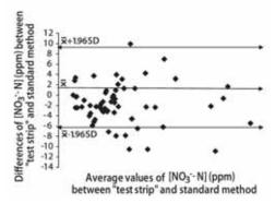
**Figure 2.**  $[NO_3^- - N]$  (ppm) differences between the methods vs. average values of the methods for each composite soil sample. ( $\bar{\mathbf{x}} =$  mean of the differences and SD = standard deviation).
